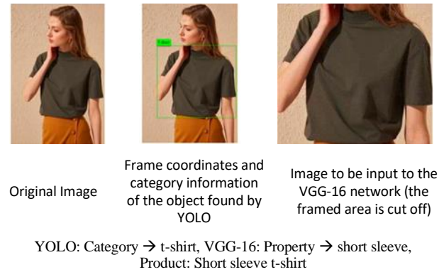
Fig. 2. Example of overdress segmentation and classification
